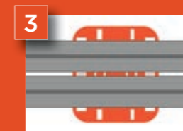
Double joists 'click' into place side by side, perfect for supporting board joints.
