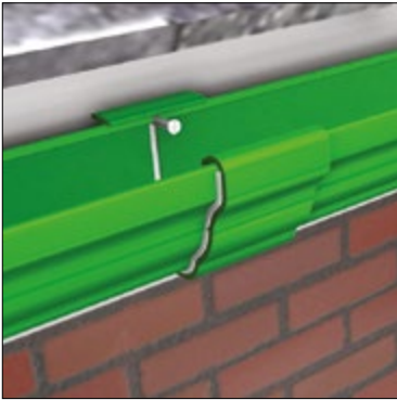
9. Anchor union to fascia board using Alutec 32mm x No. 10 screw, code SC202 or Alutec 15mm x No. 10 countersunk screw, code SC203 if fixing to Alutec aluminium composite fascia. Ensure a 3-4mm expansion gap is left.
