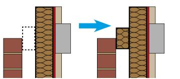
The support fixing should now be pressed through Rocksilk® RainScreen FFCB and Rocksilk® RainScreen Slab so that it touches against the sheathing board and should sit flush on top of the top layer of bricks. Rotate the fixings so that the triangle section is flat against the brickwork.
