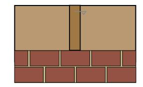
A support fixing can now be pushed through Rocksilk® RainScreen FFCB, DPC and Rocksilk® RainScreen Slab so that it sits against the sheathing board and sits halfway through the depth of the brick.
