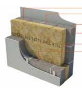
Block density: 600 to 800kg/m<sup>3</sup> Cavity width: 100mm (min)
