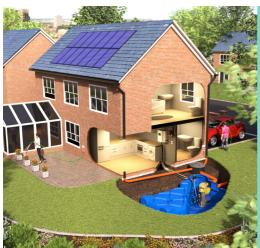
With the average home owner using around 150 litres of water per day, the StormSaver Rainwater Harvesting System will enable the metered home owner to recycle rainwater and potentially reduce their bills by up to 50%, whilst remaining kinder to the environment. StormSaver can also alleviate pressure on local drainage in line with Sustainable Drainage Schemes (SuDS), to help prevent flood risk.
