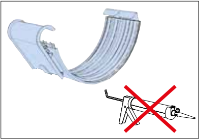
Use self sealing RSK gutter joint. Silicone should not be used.
