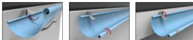
The stop end RG is self sealing. Use a rubber hammer to fix it to the gutter.
