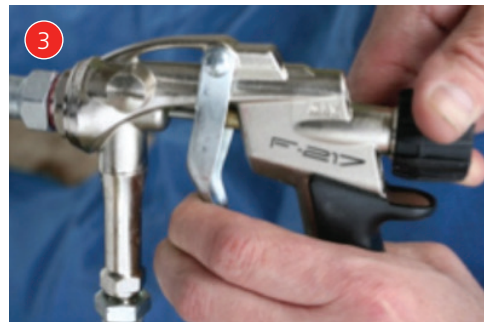
Black valve to adjust bead width.
