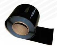
Pressure Sensitive (P.S.) Uncured Flashing Tape is a nominal 1.5mm thick, uncured, EPDM membrane laminated to a nominal 0.76mm thick, fully cured pressure-sensitive adhesive, the flashing membrane is easily malleable and highly adaptable to irregular shapes and surfaces.
