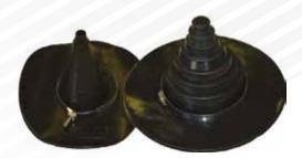
FIX-R Pressure Sensitive (P.S.) Pipe Seals are cured, pre-moulded EPDM flashing that are available in two sizes. Small Pipe Seals are for pipes from 12.5 to 75mm ( $^{1}/_{2}$ " to 3") in diameter. The larger Pipe Seal is for pipes 25 to 152mm (1" to 6") in diameter.
