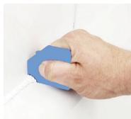
Tools can be cleaned in WHITE SPIRIT or Bond It MULTI-WIPES prior to curing taking place.
