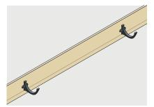
Use a string line to set out brackets to a fall of 1:600 to 1:350 (max) or if not possible, level.
