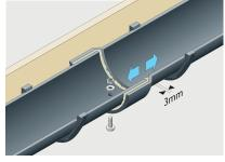
Insert the spigot end of the gutter allowing a 3mm expansion gap. Secure joint using bright zinc plated, mild steel M6 x 25mm nut, bolt and washer provided. (Bolt head preferably to underside).
