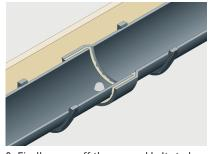
Finally, cone-off the exposed bolt stud and nut inside the gutter with a generous application of silicone sealant. Tool off excess silicone around the joint and from external surfaces.
