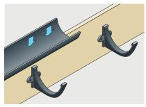
Lower the gutter onto the brackets ensuring sufficient clearance for the gutter joint. Clip gutter into bracket.
