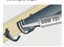
Apply two 6mm beads of DOW 791 silicone sealant either side of, and around the fixing hole.
