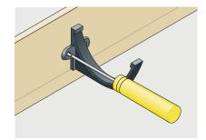
Generally, position brackets at 915mm centres allowing additional brackets on either side of where gutter joints will occur.
