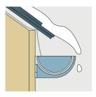
Fix brackets so as to position the gutter centrally and as close below the roof edge as possible, taking into consideration locality and roof slope finish.
