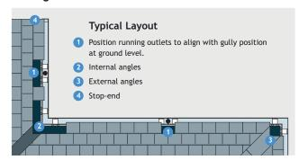
After setting out angles and outlets, fit gutters and brackets according to installation procedures for the specific rainwater system being used, as detailed in this brochure.
